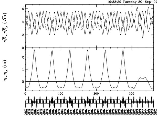
Figure 2: Beam optics functions of one superperiod of the JHF 50 GeV main ring.
