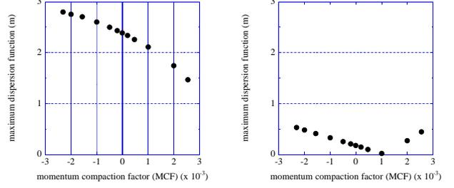
Figure 4: Maximum dispersion in the arc(left) and straight section(right) vs momentum compaction factor.
