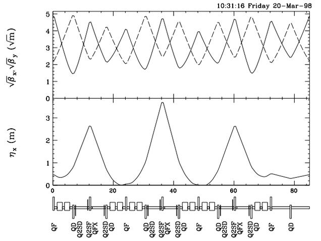
Figure 5: FMC lattice for the 3 GeV booster.
