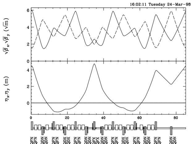
Figure 6: FMC lattice for the 6 GeV booster.
