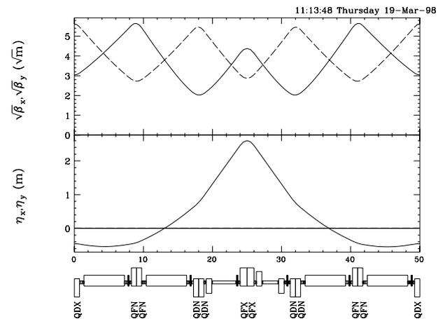
Figure 1: Beam optics functions of the module in arc section of the JHF 50 GeV main ring.  $\beta_x^{1/2}$ :solid line,  $\beta_y^{1/2}$ :dashed line.
