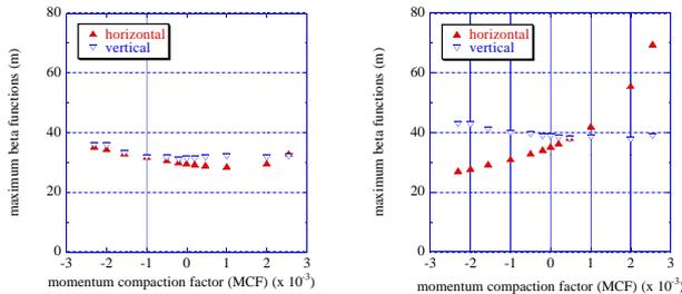
Figure 3: Maximum beta in the arc(left) and straight section(right) vs momentum compaction factor.
