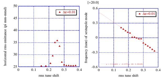
Figure: 6 (a) Emittance growth and (b) coherent tune of sextupole when the test lattice has sextupole field errors.
