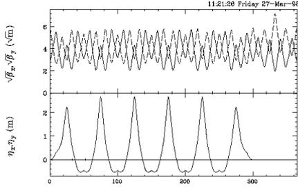
Figure: 2 Lattice functions with dispersion suppressor.
