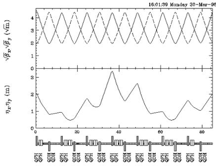
Figure: 5 Lattice functions of a quarter of the booster.
