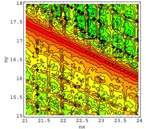
Figure: 4 Dynamic aperture with one missing sextupoles.
