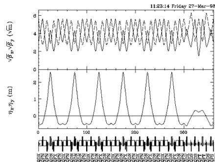
Figure: 1 Lattice functions of a quarter of the main ring.
