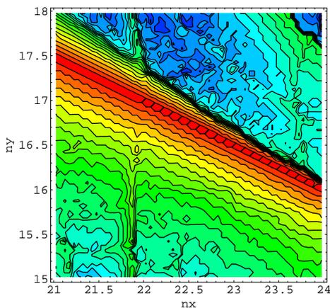
Figure: 3 Dynamic aperture surveyed in 2-D tune space. The darkest gray means zero aperture and the lightest one four times as much as the physical aperture in size.
