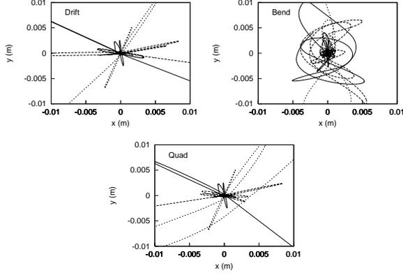
Figure 1: Trajectory of ions in drift space, bending and quadrupole magnetic field. Three ions with different initial random seeds are tracked.
