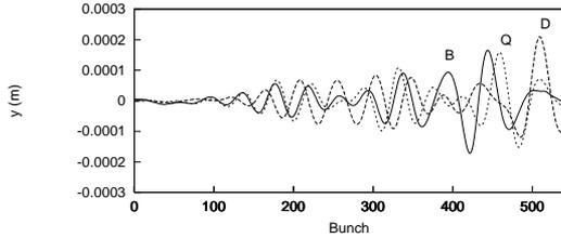
Figure 3: Bunch correlation pattern after 1000 revolutions. Vertical bunch amplitudes observed at a position in the ring are plotted.
