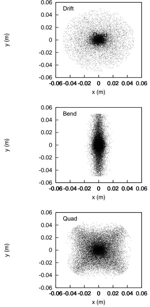
Figure 2: Equilibrium distributions of ions in drift space, bending and quadrupole magnetic field.
