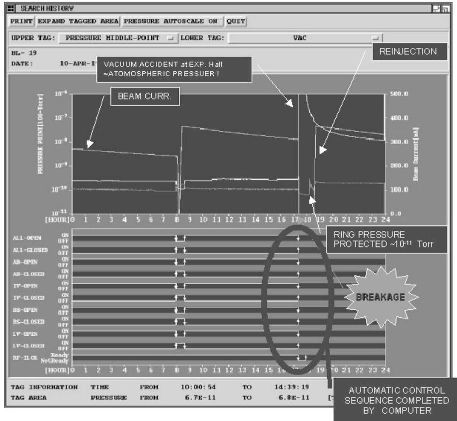
Fig.2 Retrieval result generated by the archiving system to inspect whether two accelerator components are functioning properly.
