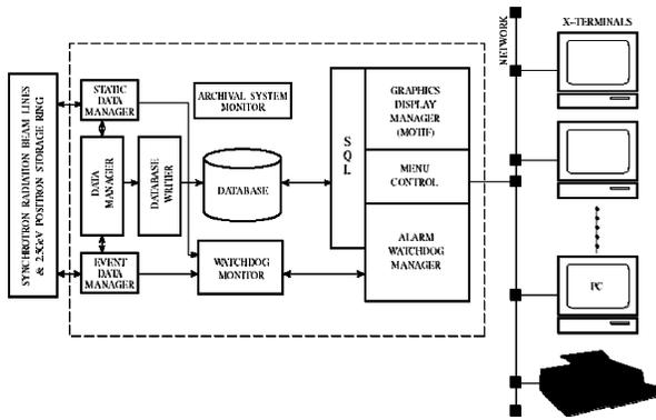
Fig.1 Block diagram of the archiving system for high energy accelerator components.
