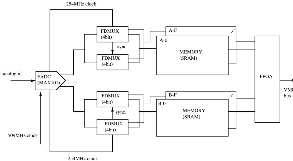
Figure 2: Block-diagram of the memory board. The signal which holds the bunch-current information is digitized with the ADC in rate of 509MSamples/s. The ADC outputs the digitized data from two output ports each of them has the 254MHz rate. These signals are de-multiplexed by the custom LSIs. One chip of the de-multiplexer can treat 4-bit data. The de-multiplexed data are stored in 16 identical memory banks.
