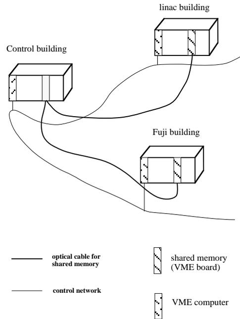
Figure 3: Distribution of the bunch-current information with the shared memory system. Besides the standard control network, the three computers are connected with the dedicated communication system through the optical fiber cables.
