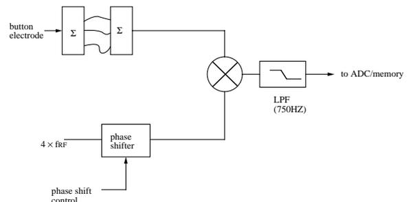
Figure 1: Front-end circuit of the bunch-current measuring system. The two combiners/splitters and three cables make a band-pass filter. The differences in the lengths of the shortest cable and the other two cables are the wavelength of 2GHz and twice of it.
