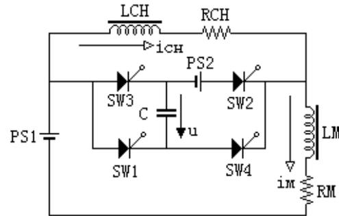
Fig.1. Fundamental Principle of the SRMPS
