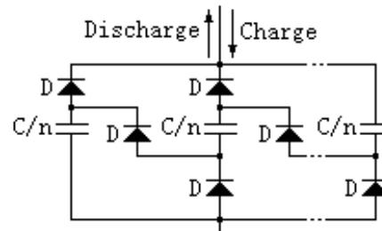
Fig. 2: Diagram of Discharge /Charge of n (C/n) s in Series/Parallel
