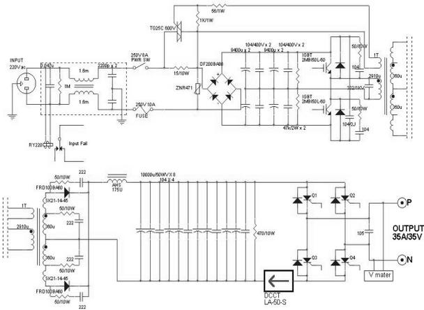
Figure 2. Main Circuit of Developed Prototype MPS
