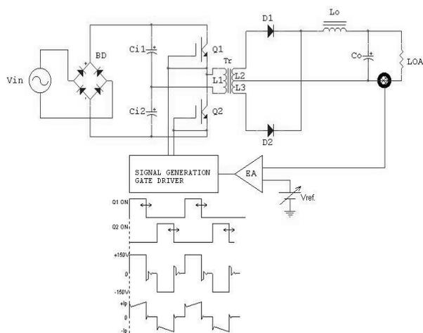
Figure 1. Main Circuit Concept
