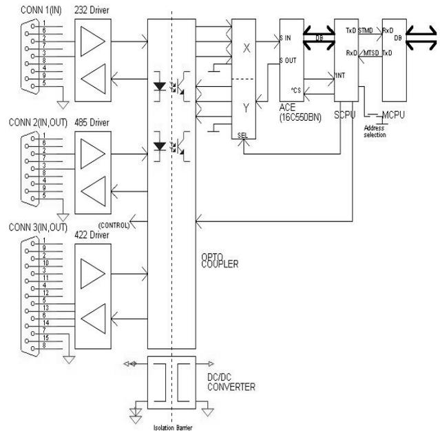
connection by one driver method. By half-duplex method, RS485 can be used for one to thirty two connection at the maximum. By full-duplex method, RS422 can be used for one to ten connection at the maximum. In case of RS485 or RS422, address of each MPS is inputted in MCPU by key pad of front panel.
