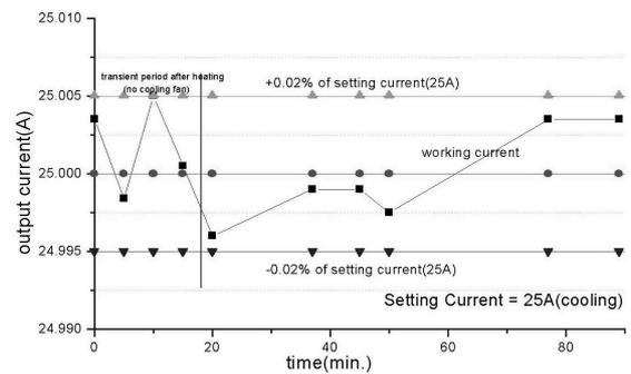
Figure 7. Output Current Stability of Prototype MPS
