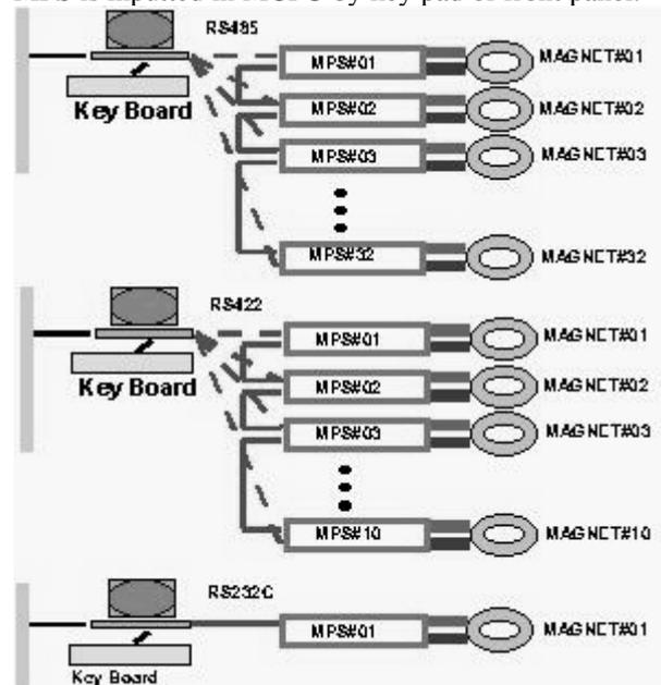
Figure 3. Block Diagram of Remote Controller Serial Communication
