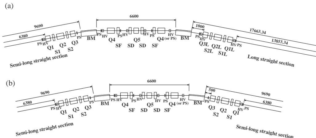
Figure 1: Layout of the ring magnets for (a) Long Cell and (b) Normal Cell.
