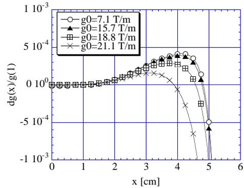
Figure 5: Field gradient uniformity of the quadrupole.
