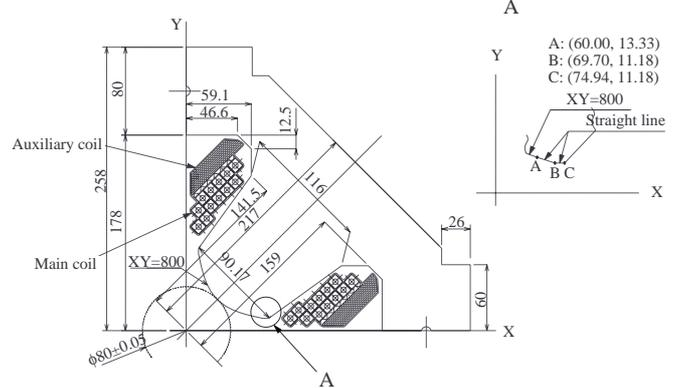
Figure 4: The quadrupole magnet.
