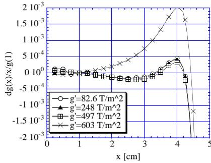
Figure 7: Field gradient uniformity of the sextupole.
