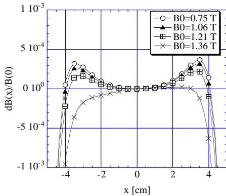
Figure 3: Field uniformity of the dipole.
