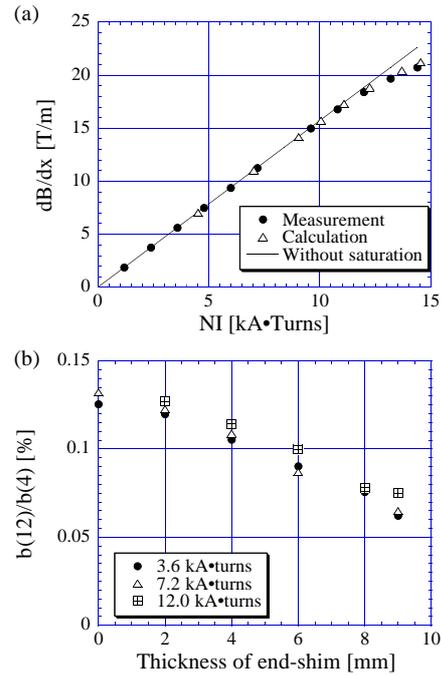
Figure 8: Preliminary results of the field measurement for the quadrupole prototype; (a) excitation curve, (b) relation between thickness of end-shim and normalized dodecapole component at 30 mm from magnet center.
