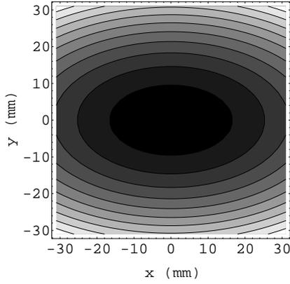
Fig. 2 Contour plot of  $B_y$  for the helical dipole, with  $b_1=1$ , and  $b_3, b_5, \dots=0$ .
