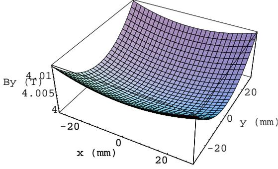
Fig. 1 3D plot of  $B_y$  for the helical dipole, with  $b_1=1$ , and  $b_3, b_5, \dots=0$ .
