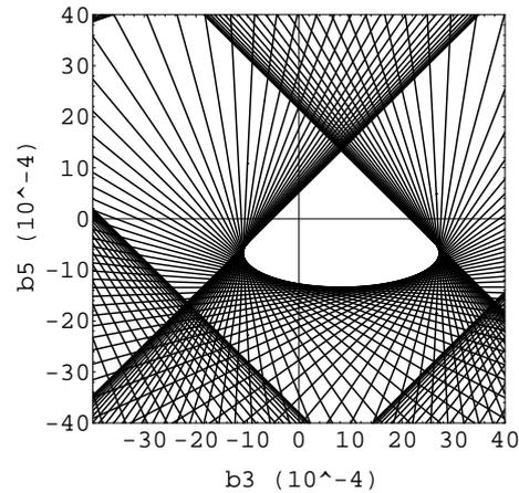
Fig. 8  $(b_3, b_5)$  relation of  $< 0.3$  % of  $|B_y - B_{y0}|/B_{y0}$  with  $b_7=0$ , and  $b_9, b_{11}, \dots=0$ .
