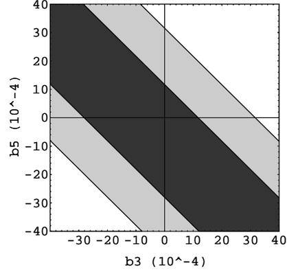
Fig. 6  $(b_3, b_5)$  relation of  $< 0.2$  % and  $< 0.4$  % of  $|B_y - B_{y0}|/B_{y0}$  at ( $x = 31$  mm,  $y = 0$  mm) with  $b_7=0$ , and  $b_9, b_{11}, \dots=0$ .
