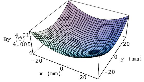
Fig. 3 3D plot of  $B_y$  for the helical dipole with  $b_1=1$ ,  $b_3=0.00082$ , and  $b_5, b_7, \dots=0$ .
