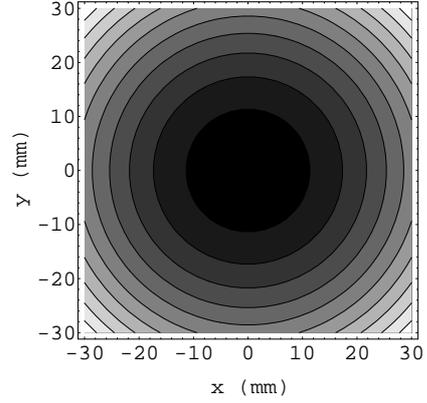
Fig. 4 Contour plot of  $B_y$  for the helical dipole, with  $b_1=1$ ,  $b_3=0.00082$ , and  $b_5, b_7, \dots=0$ .
