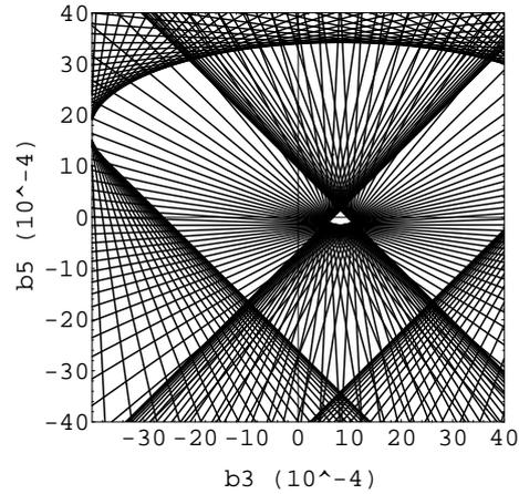
Fig. 7  $(b_3, b_5)$  relation of  $< 0.18$  % of  $|B_y - B_{y0}|/B_{y0}$  with  $b_7=0$ , and  $b_9, b_{11}, \dots=0$ .
