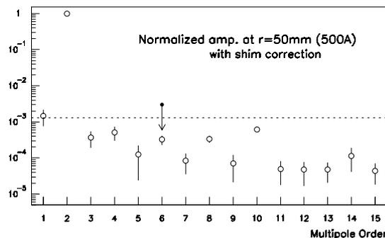
Figure 8: Normalized multipole amplitude plotted as a function of multipole order for Qarc(LER) magnets. The solid circle indicates the 6th multipole before the correction. The requirement for the lowest allowed multipole ( $n=6$ ) is indicated by a dotted line. The error bars indicate one standard deviation of each multipole.
