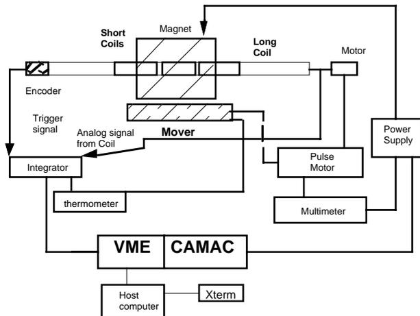
Figure 1: Schematic diagram of the field measurement system. A mover is used for adjusting the magnet position with respect to the measurement system (not shown).
