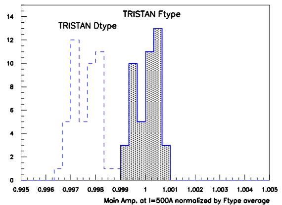
Figure 5: The main amplitude (normalized by the TRISTAN F-type average) distribution at I=500A. TRISTAN F-type and D-type magnets correspond to the upper and the lower peaks, respectively.
