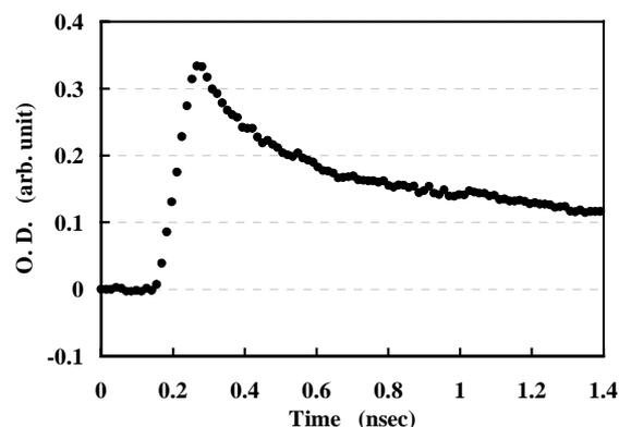
Fig. 3 Time-dependent behavior of the n-dodecane cation radical obtained in the picosecond pulse radiolysis of n-dodecane monitored at 820 nm.
