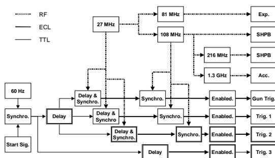
Fig. 2 Rf and Triggering system
