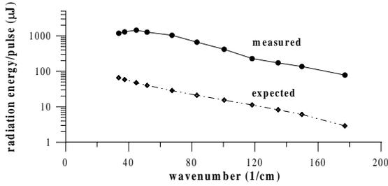
Figure 6: Measured and expected radiation energy per pulse vs. wavenumber
