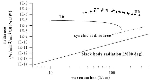
Figure 8: FIR radiation obtained from f-sec electron bunches compared with black body radiation and synchrotron radiation
