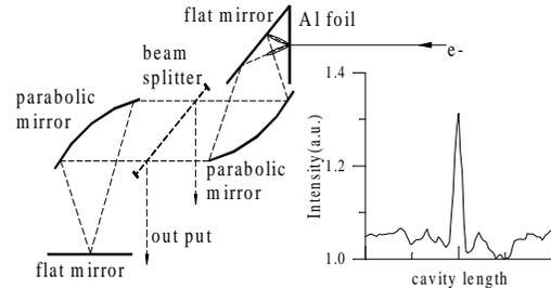
Figure 5: The STR cavity and intensity vs. cavity length
