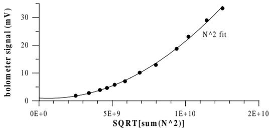
Figure 2: TR intensity as a function of beam current<sup>1</sup>
