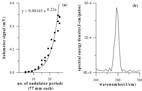
Figure 7: Exponential growth of UR at 53 μm due to SASE[6,7] (a) and spectral distribution (b)
