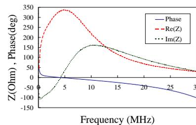
Figure 3: Impedance of the HG cavity.
