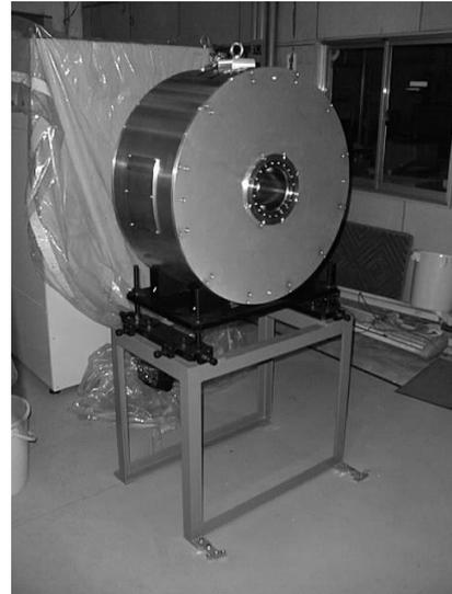
Figure: 2 High Gradient RF cavity. A 200 kW class push pull amplifier will be located under the cavity.
