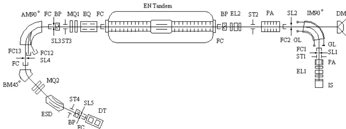
Fig.1. Schematic layout of the AMS facility in Peking University
