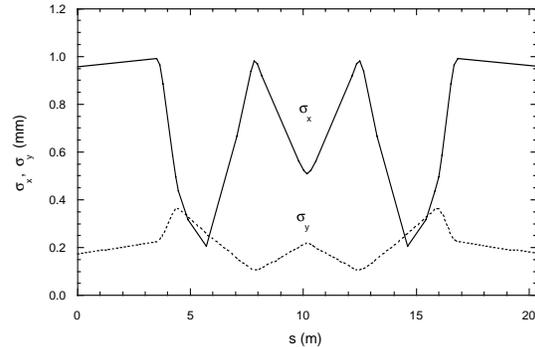
Fig. 3. Beam sizes in a unit cell. 10 % coupling is assumed.
