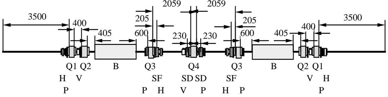
Fig. 1. Magnet arrangement in a quadrant of the storage ring. B: bending magnet, Q1~Q4: quadrupole magnet, SF and SD: sextupole magnets, H: horizontal steerer, V: vertical steerer, and P: position monitor. The distances are shown in mm.
