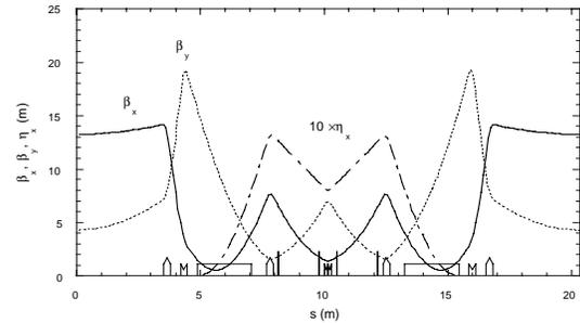
Fig. 2. Betatron functions and the dispersion in a unit cell.
