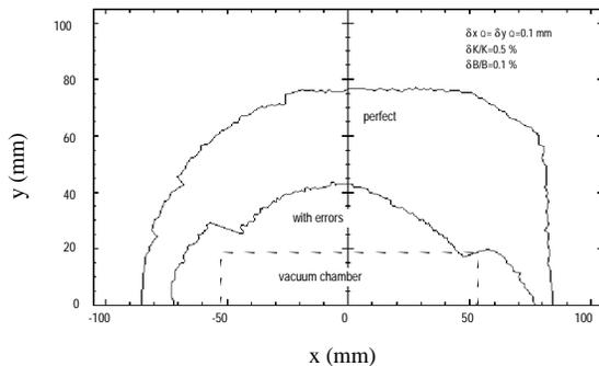
Fig. 4. Dynamic apertures for a perfect machine and a realistic machine with errors.
