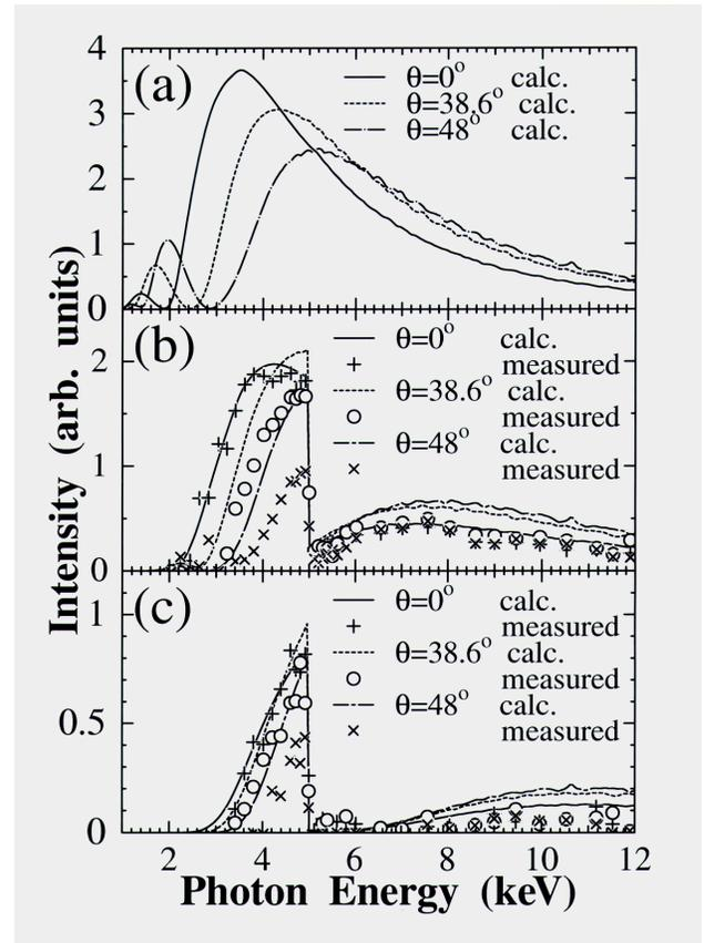
Fig. 1: The calculated and measured transition radiation spectra from the 1-GeV electron beam incident on the eight-foil stack of 7.5- $\mu\text{m}$  thick Kapton tilted at  $\theta=0^\circ$ ,  $38.6^\circ$ ,  $48^\circ$ ; (a) without the titanium filter (the calculated results only), (b) with the 8- $\mu\text{m}$  titanium filter, (c) with the 28- $\mu\text{m}$  titanium filter.
