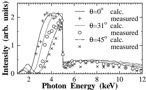
Fig. 2: Same as Fig. 1 for the 3- $\mu\text{m}$  thick titanium eight-foil stack tilted at  $\theta=0^\circ$ ,  $31^\circ$ ,  $45^\circ$ .
