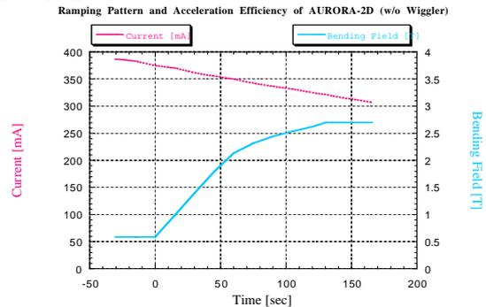
Fig. 4-a) Typical acceleration pattern of A2D.
