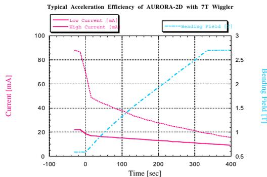
Fig. 4-b) Acceleration efficiency of A2D with wiggler.
