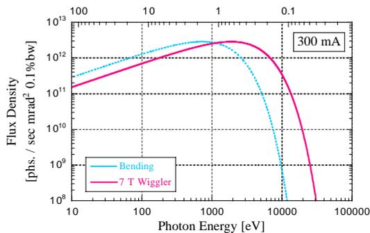
Fig. 3 Energy spectra of SR from 7 Tesla wiggler.
