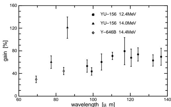
Figure 3: FEL gain as a function of the wavelength above 50  $\mu\text{m}$ . The gain values denoted by the circles and the triangles were obtained at an electron energy of 12.4 and 14.0 MeV using the electron gun YU-156, respectively, and the open diamonds were obtained at 14.4 MeV using the electron gun Y-646B.
