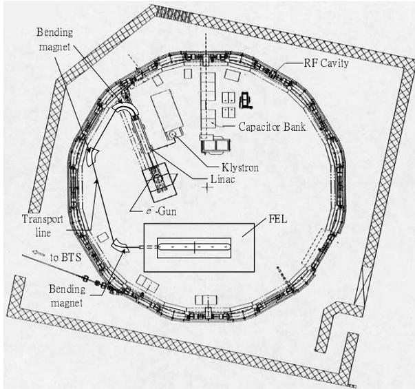
Fig. 1 Layout of the Linac, synchrotron booster and the FEL.
