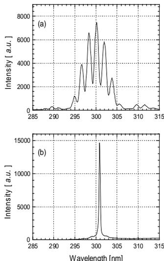
Fig. 1 Output spectra of spontaneous emission(a) and lasing (b). The deflection parameter is 2.0.
