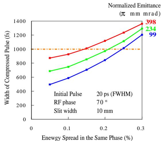
Fig.3 Relation between beam quality and width of compressed pulse
