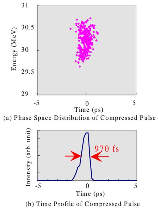
Fig. 4 Calculated longitudinal phase space distribution of compressed pulse
