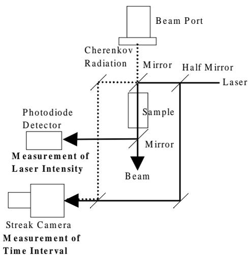
Fig. 6 Jitter compensation system for pulse radiolysis.
