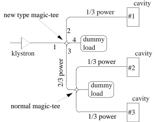
Figure 1. Block diagram of the RF power-source system
