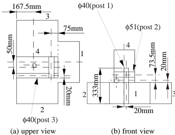
Figure 5 Optimal design of the new type magic-tee
