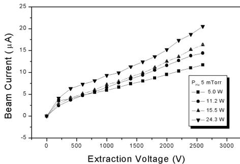
Fig. 7 Extracted beam currents as a function of RF power at various gas pressure.
