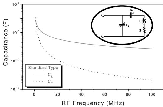
Fig. 2 A circuit diagram for the matching box and the plot of capacitors in the box for the 1" diameter antenna.
