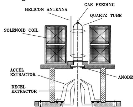
Fig. 8 A new design of helicon ion source.
