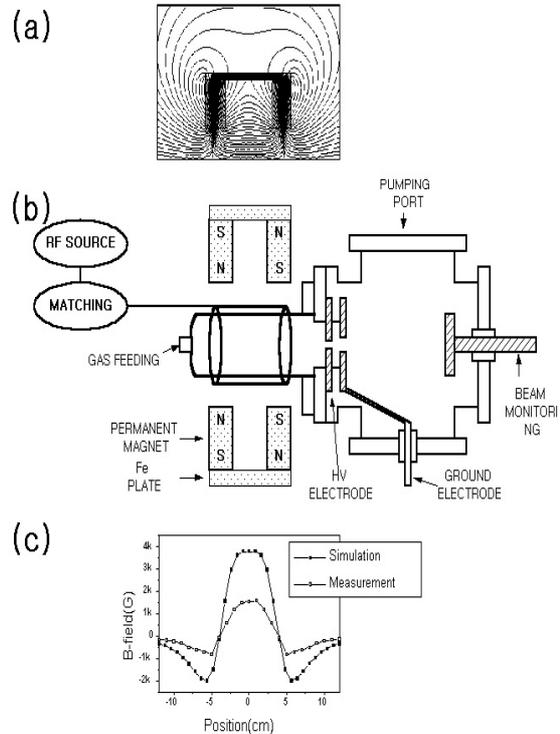
Fig. 4 Arrangement and magnetic field structure of the permanent magnet for the compact helicon source.
