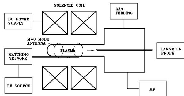
Fig. 1 Schematic of the helicon plasma source.
