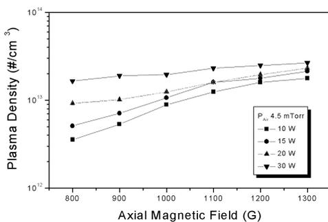
Fig. 3 Plasma density variation with respect to RF power and magnetic field strength.
