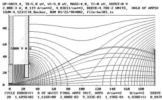
Fig. 6 Extracted beam profiles simulated by IGUN code.
