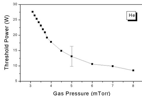
Fig. 5 Threshold powers of the helicon plasmas at various gas pressure.
