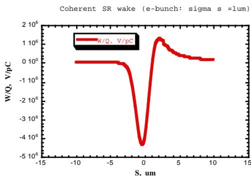
Fig. 3 Coherent SR Wake-field for electron bunch with RMS bunchlength of 1 micron.
