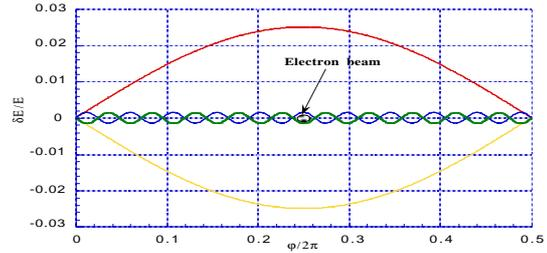
Fig.2 . A combination of long wavelength RF and short wavelength RF provide both large energy acceptance and strong focusing.
