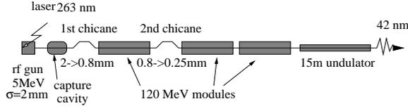
Figure 3: Beamline layout of the TTF VUV FEL phase I
