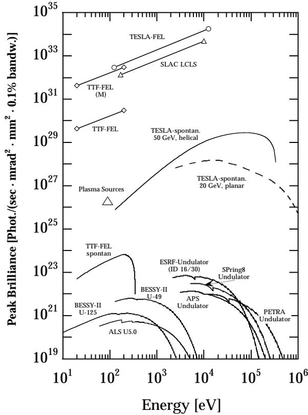
Figure 1: Spectral peak brilliance of XFELs based on the TESLA linear collider, together with that of third generation synchrotron radiation sources and the LCLS project discussed at SLAC, Stanford, USA [8]
