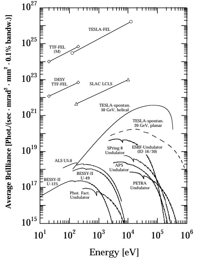
Figure 2: Spectral average brilliance of XFELs and various third generation synchrotron radiation sources
