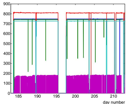
Figure 12: Cavity voltages (in kV) during July 2004. New cavity: 810 kV, old cavities:  $\sim 740$  kV). Beam current (in  $\mu A/10$ )
