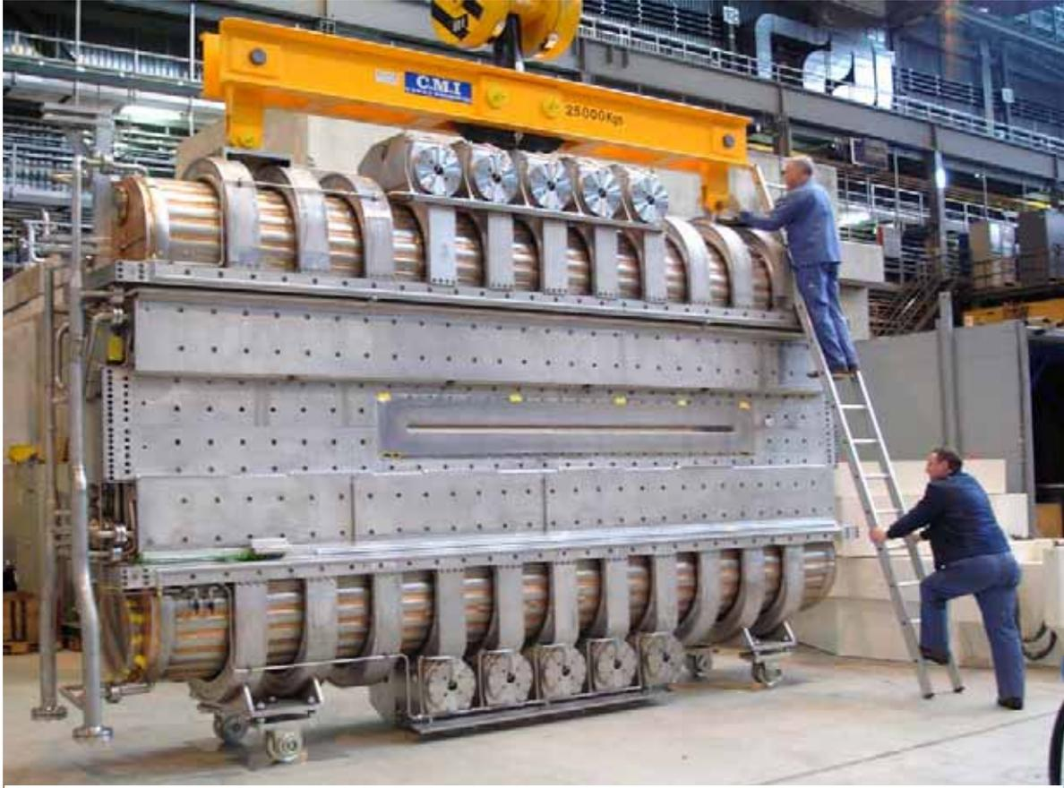
Figure 9: Completed cavity in the experimental hall at PSI.
