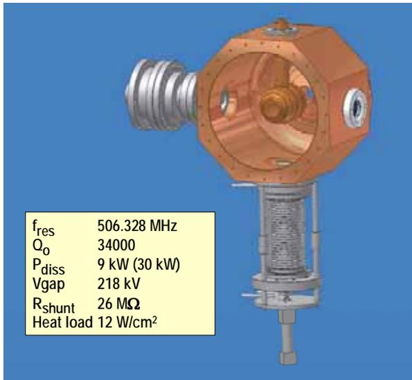
Figure 2: CAD model (with front cover removed) of a Rebuncher at the 10<sup>th</sup> Harmonic.
