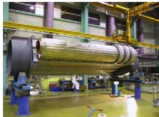
Figure 7: Mounting the yokes.
