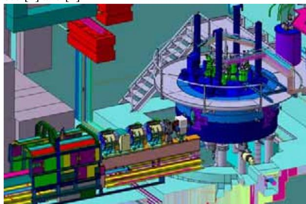
Figure 1: Superconducting cyclotron for Proscan
