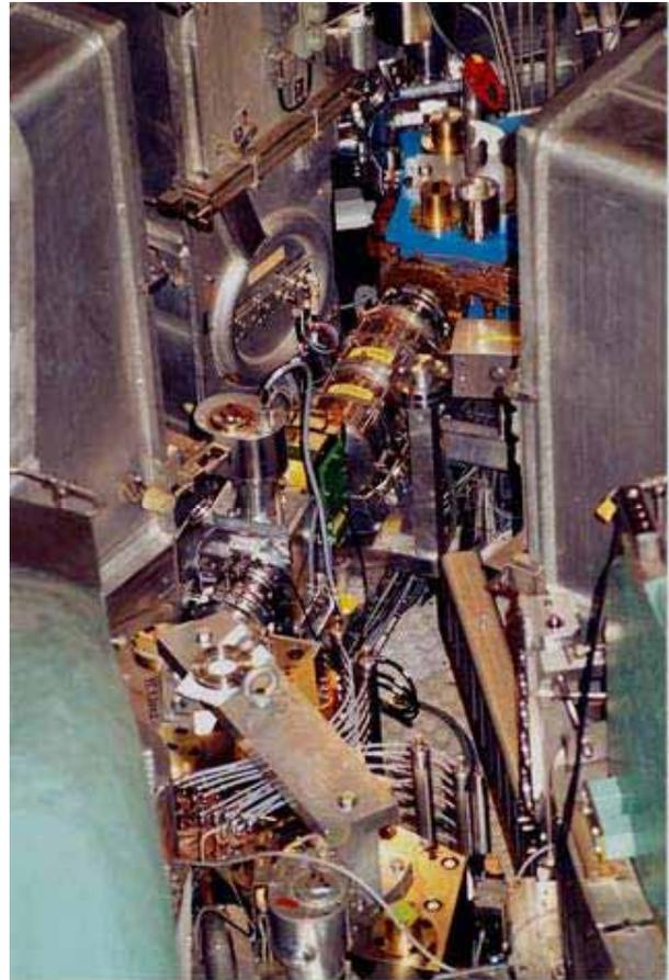
Figure 4: Beam line section in the centre of the 590 MeV cyclotron
