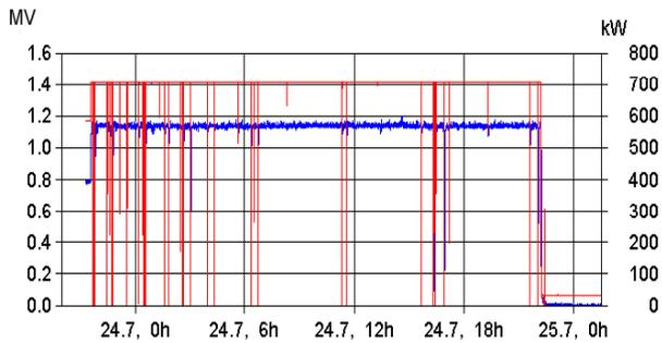
Figure 10: Gap voltage ( $R_{sh}=1.7M\Omega$ ) and dissipated power (570 kW) during the site acceptance test.
