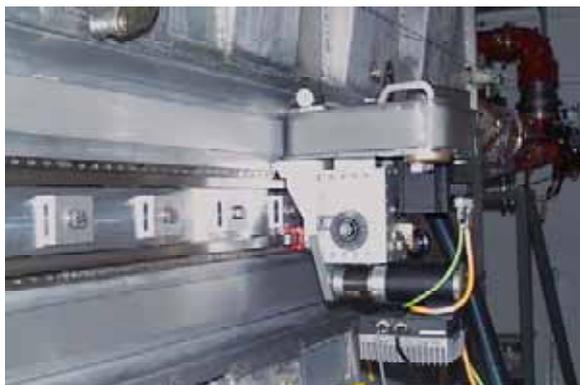
Figure 3: Grinder/polisher module
