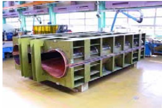
Figure 6: Copper shell in the welding jig.
