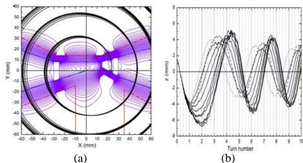
Figure 3: (a) Horizontal trajectories of the ions (b) Vertical trajectories of the ions
