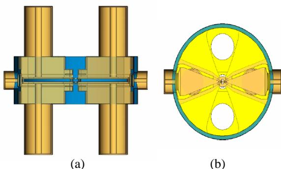
Figure 6. (a) Cross-sectional view of the cavities (b) Cross-sectional view of Dees in the mid-plane.
