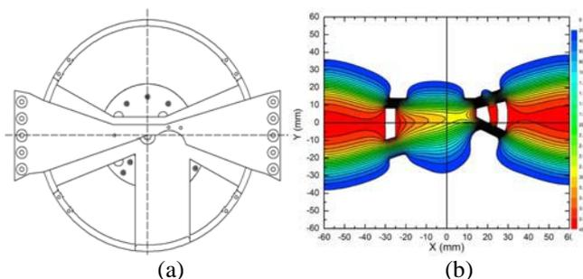
Figure 2: (a) New design of central region. (b) Electric potential map
