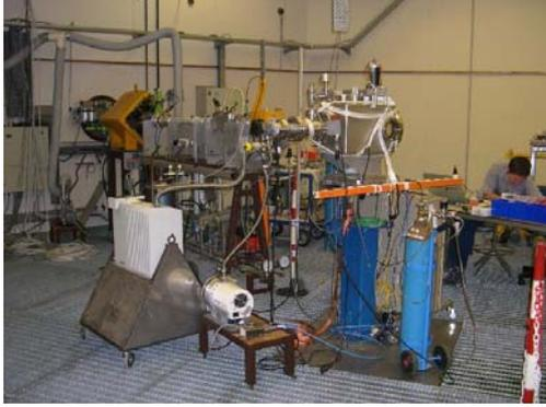
Figure 2: The SLIM beam monitor installed on a JRC Cyclotron beam line.
