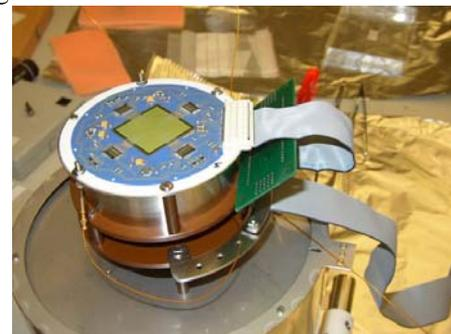
Figure 5: Pad detector hybridized on ceramic and mounted at the end of the SLIM focusing system.
