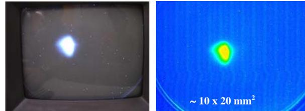
Figure 4: Beam profile measured with the SLIM; left, the CCD signal on a video monitor, right, digitised with a frame grabber.
