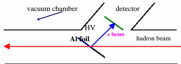
Figure 1: Schematic layout of the SLIM beam monitor.
