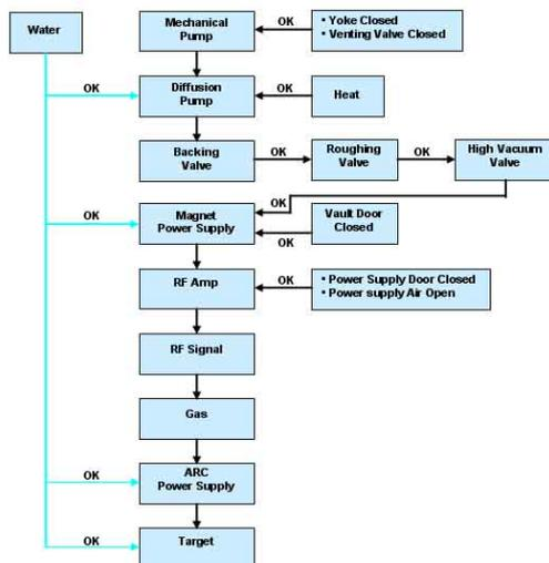
Fig.4 Interlock System Layout
