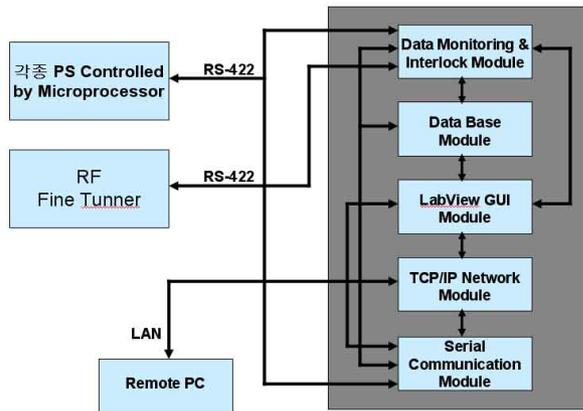
Fig.3 Distributed Control System of KIRAMS-13
