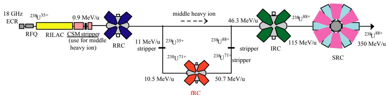
Fig.1 : Acceleration scheme in the RIBF
