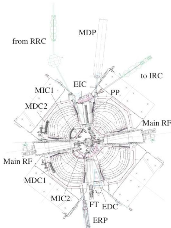
Fig. 2: Layout of the fRC.
