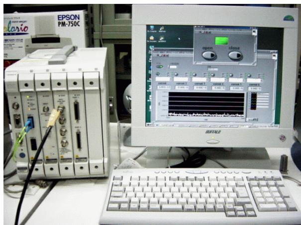
Figure 4: A picture of the WE7000 station and the Labview programs for beam current measurements.
