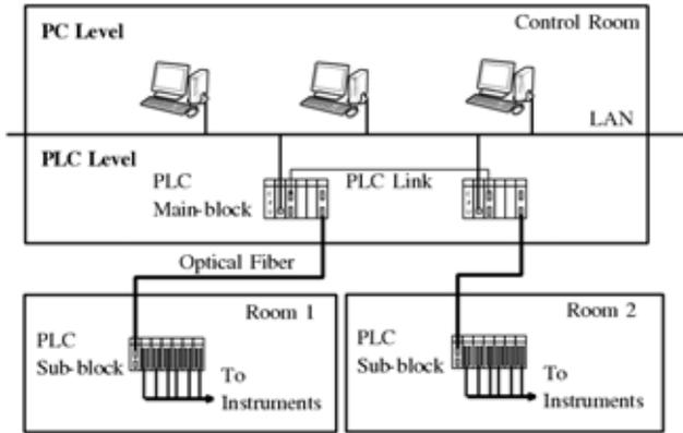
Figure 1: A schematic view of the control system.
