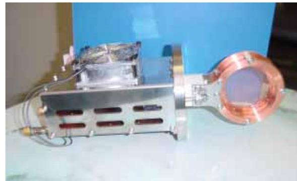
Figure 3: A picture of the electrodes of the beam buncher.
