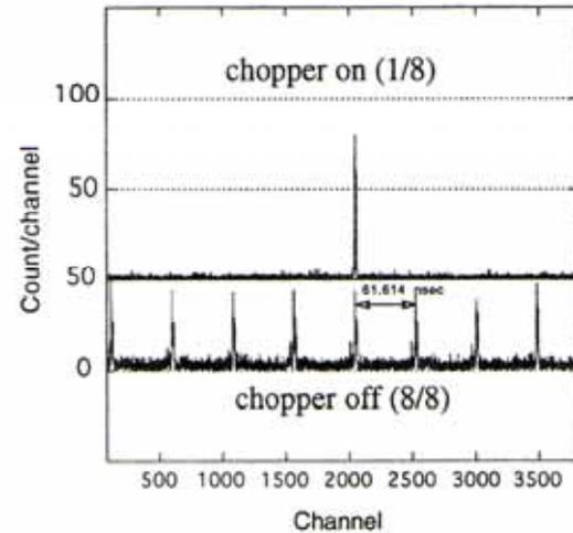
Figure 2: Result of performance test for the sinusoidal beam chopper, by which unwanted micro-bursts of the beam are removed from the beam-line.
