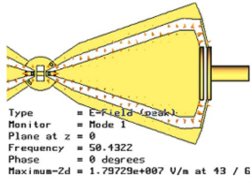
Figure 8: The electric field distribution in the mid-plane.
