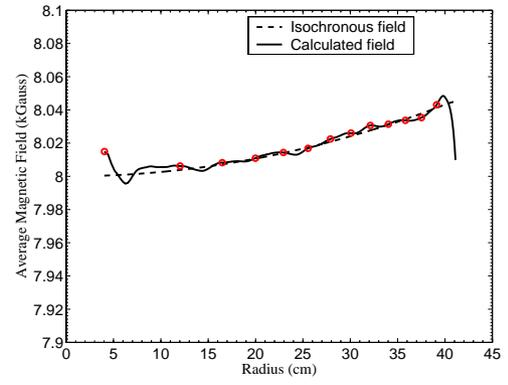
Figure 2: Average magnetic field with the radius at median plane.
