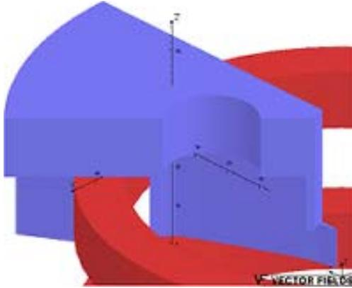
Figure 1: 1/8 designed model of the magnet.
