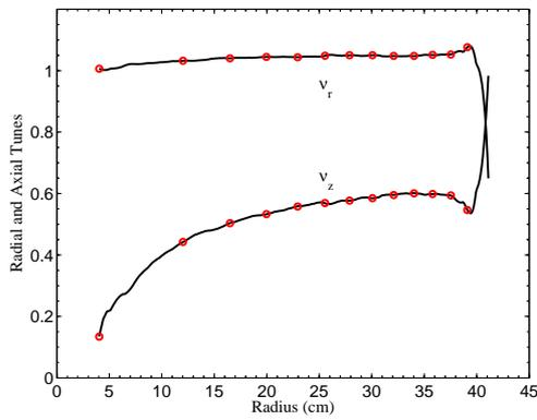
Figure 5: Radial and axial tunes with the radius.
