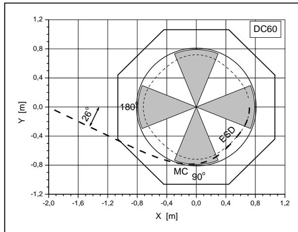
Figure 3: The scheme of the beam extraction.
