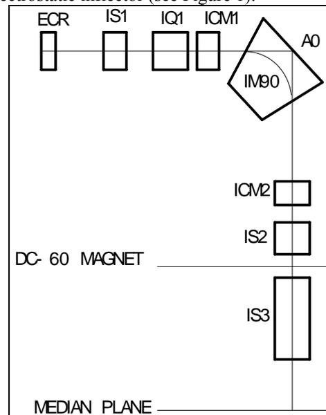
Figure 1: Scheme of axial injection channel. IS1, IS2, IS3 - focusing solenoids. IM90 - analyzing magnet. IQ - quadrupole lens, ICM1, ICM2 correcting magnets.
