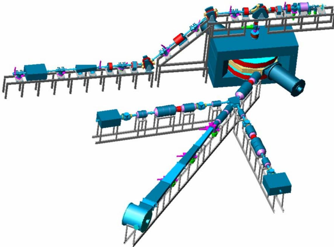
Figure 4: The layout of the DC-60 cyclotron with transported channels.
