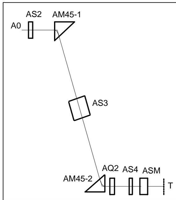
Figure 2: Scheme of the channel for applied research. AS2 ÷ AS4 - focusing solenoids, AM45-1, AM45-2 - 45° bending magnets, AQ2 - quadrupole and T is a beam target.
