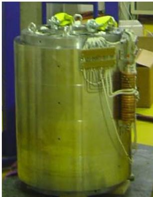
Figure 6:SECRAL superconducting magnet assembly.
