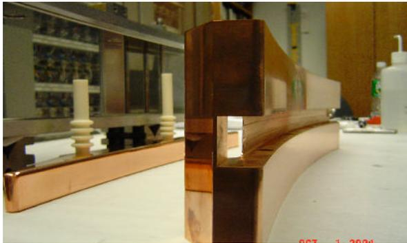
Figure 9. Current version of electrostatic deflector
