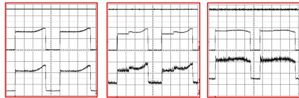
Figure 10. Beam Current Modulation Examples. The upper trace is the desired function and the lower trace is the actual cyclotron output.
