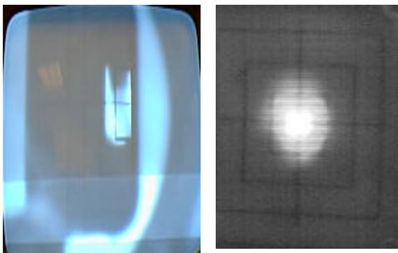
Figure 7. Extracted beam spot showing sextupole component (on left) and after focussing (on right).
