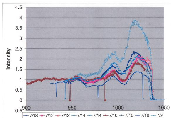
Figure 6. Several radial probe scans for different Gradient Corrector geometries in the last 10 cm of the Cyclotron radius. The vertical axis is relative intensity.
