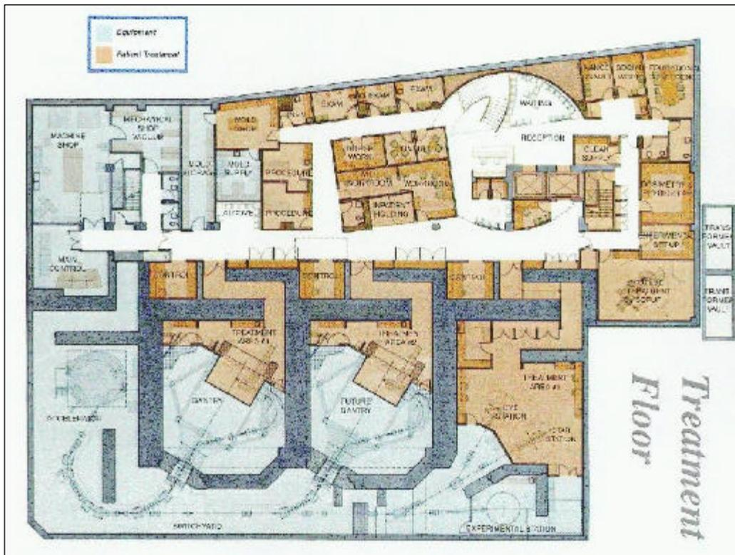
Figure 4. Physical Layout of the Northeast Proton Therapy Center. This facility includes the IBA C230 Cyclotron and Energy Selection System, Beamline, Two Gantry Treatment Rooms and a Fixed Beam Room with 3 Beamlines.
