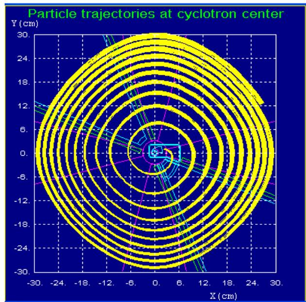
Figure 7: Ion trajectories in the central region
