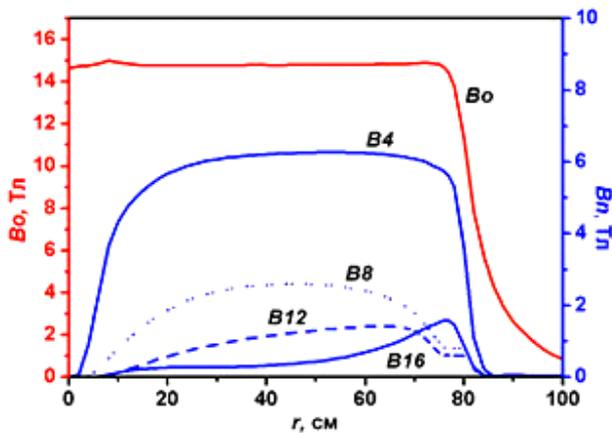
Figure 3: Cyclotron magnetic field
