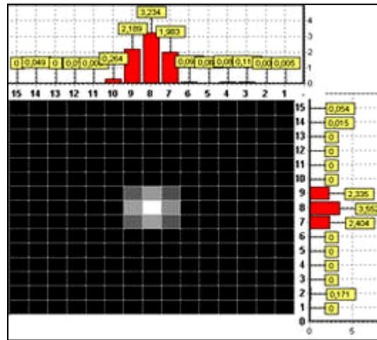
Figure 4: Beam profile in injection line
