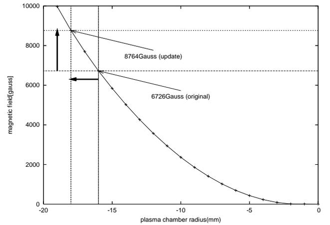
Figure 4: The calculated magnetic field distribution of radial direction in the plasma chamber using the OPERA-3D code.
