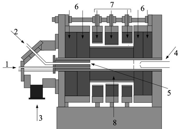
Figure 1: Schematic view of ion source. (1) gas injection (2) microwave injection (3) 150 l/sec TMP (4) extraction electrode (5) microwave tuning panel (or magnetic stainless steel cylinder + bias electrode) (6) main ring magnet (7) additional ring magnet (8) hexapole magnet
