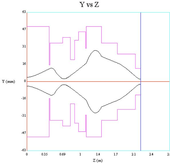
Figure 3: Vertical  $H^-$  beam profile for proposed ISIS.
