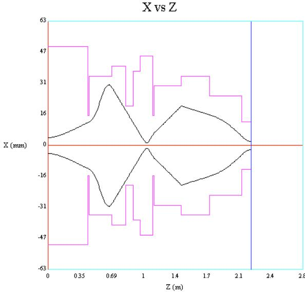
Figure 2: Horizontal  $H^-$  beam profile for proposed ISIS.
