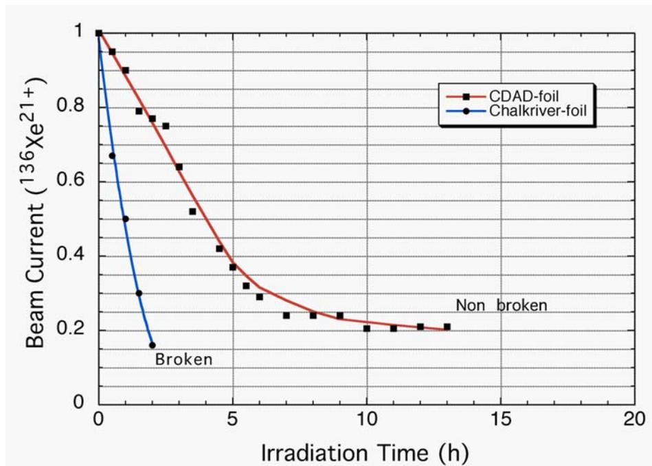
Figure 3: Relation between beam current of  $^{136}\text{Xe}^{21+}$  and irradiation time (h).
