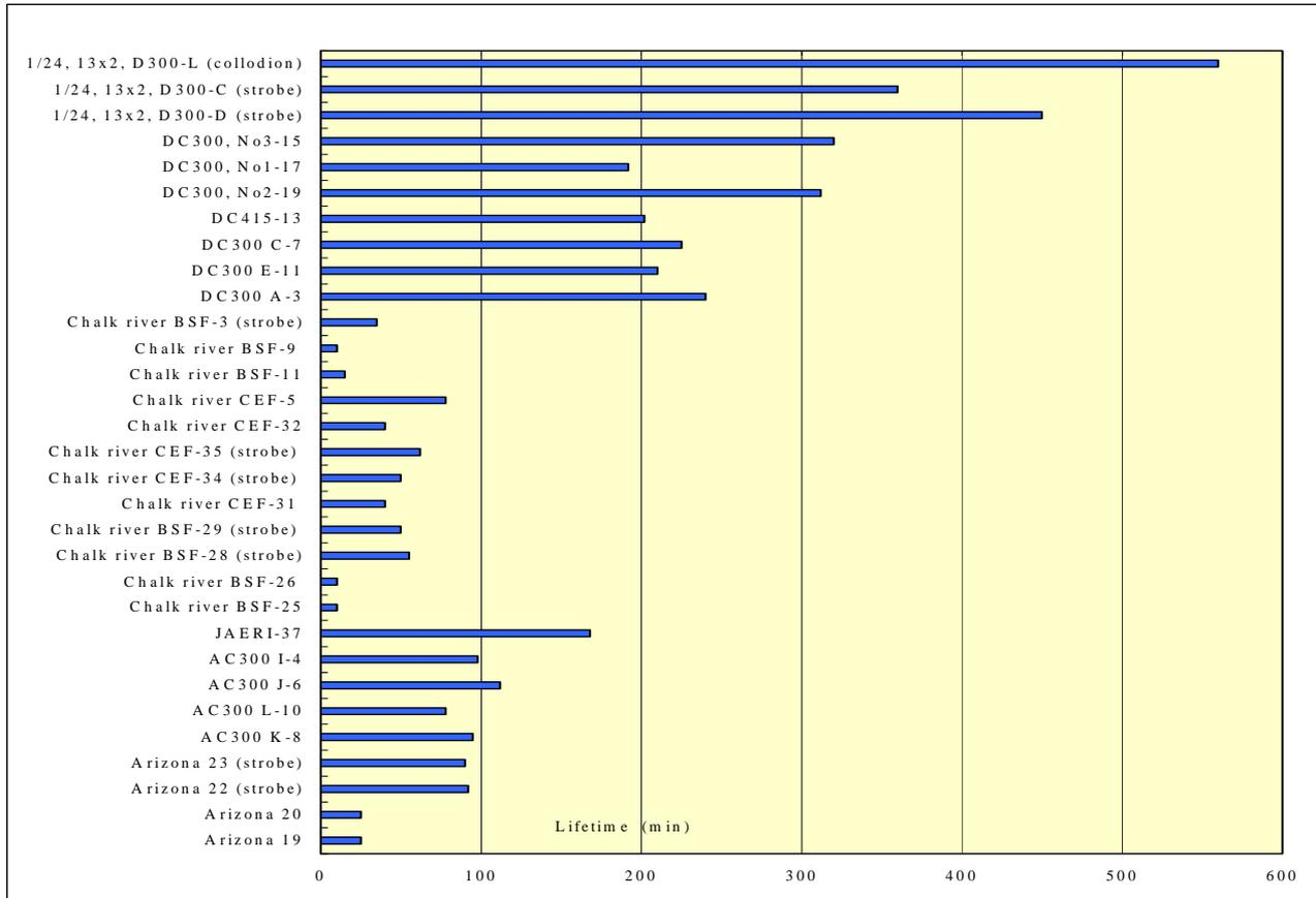
Figure 1: Comparison of the lifetimes of various carbon foils under bombardment with a 0.25 MeV/u,  $^{136}\text{Xe}^{9+}$  of 1.1  $\mu\text{A}$  and  $5 \times 5$  mm in beam spot.
