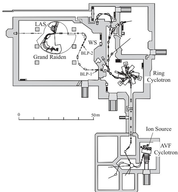
Figure 1: Layout of the RCNP cyclotron facility.
