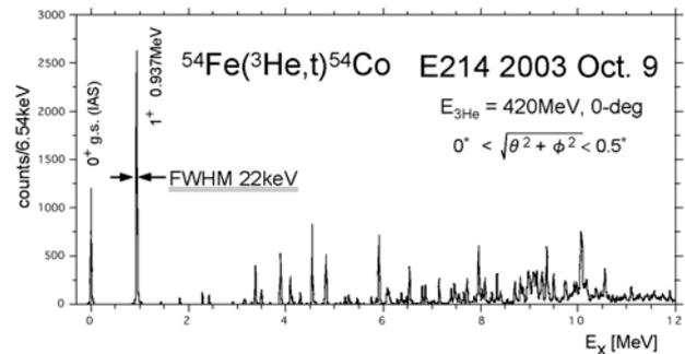
Figure 2: Excitation energy spectrum of  ${}^{54}\text{Fe}({}^3\text{He}, t){}^{54}\text{Co}$  reaction measured at 420 MeV and 0 degree.
