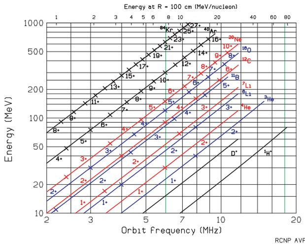
Figure:3: Resonance conditions for ion acceleration
