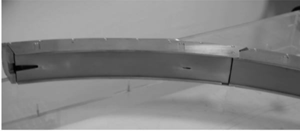
Figure 3: Damaged septum of the electrostatic deflector.
