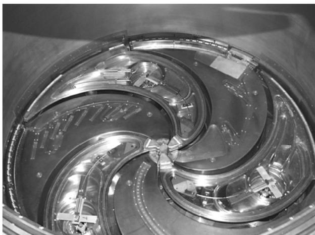
Figure 1: View of the Cyclotron median plane.
