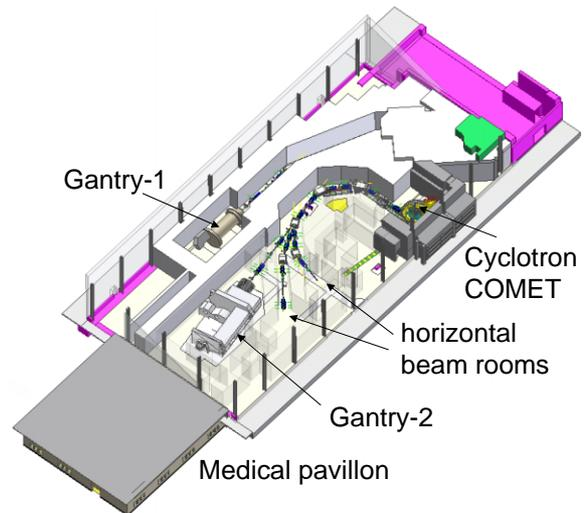
Figure 1: Layout of PSI's new dedicated proton therapy facility *PROSCAN*. Gantry-1 and Gantry-2 are the existing and the new gantry, respectively.
