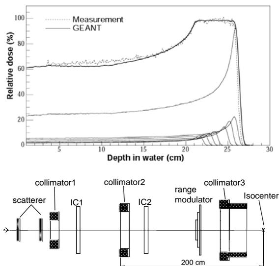
Figure 3: Formation of a 5 cm SOBP with a rotating modulation wheel and arrangement of beam-modifying elements in the horizontal fixed beam line of the MPRI.
