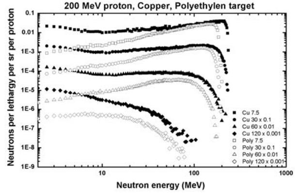
Figure 2: Neutron energy spectrums at different angles for two different target materials.
