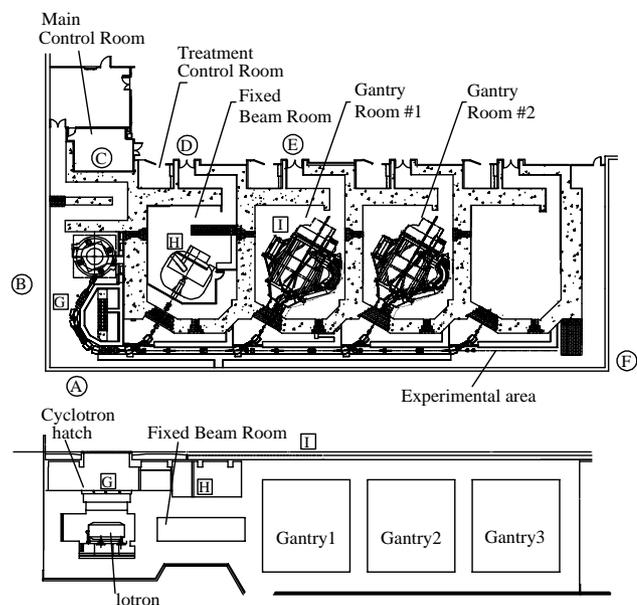
Figure 1: Layout and sectional view of the proton therapy facility.
