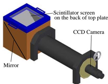
Figure 4: Schematic view of a 2D dose measurement system composed of CCD camera and scintillating screen.
