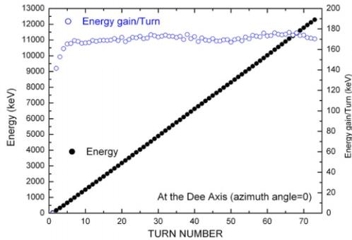
Figure 6: Energy gain/Turn and beam energy with turn number.
