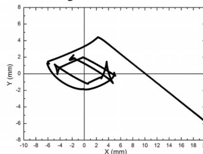
Figure 5: The motion of the center of the ion trajectory during the 2 turns.
