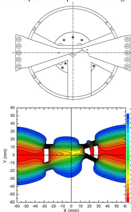
Figure 1: The CAD drawing (upper) and the electric potential map (lower) of new central region.
