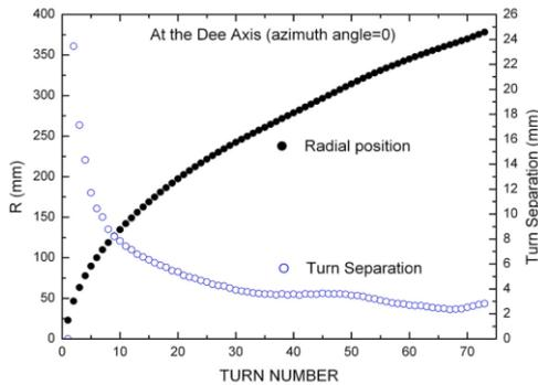
Figure 7: Turn separation and the radial position with turn number.
