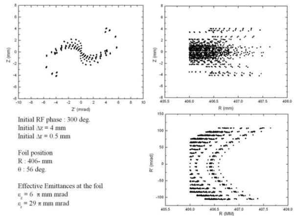
Figure 8: Beam characteristics at the extraction carbon foil.
