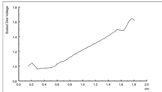
Figure 3. The distribution of the Dee voltage along gap
