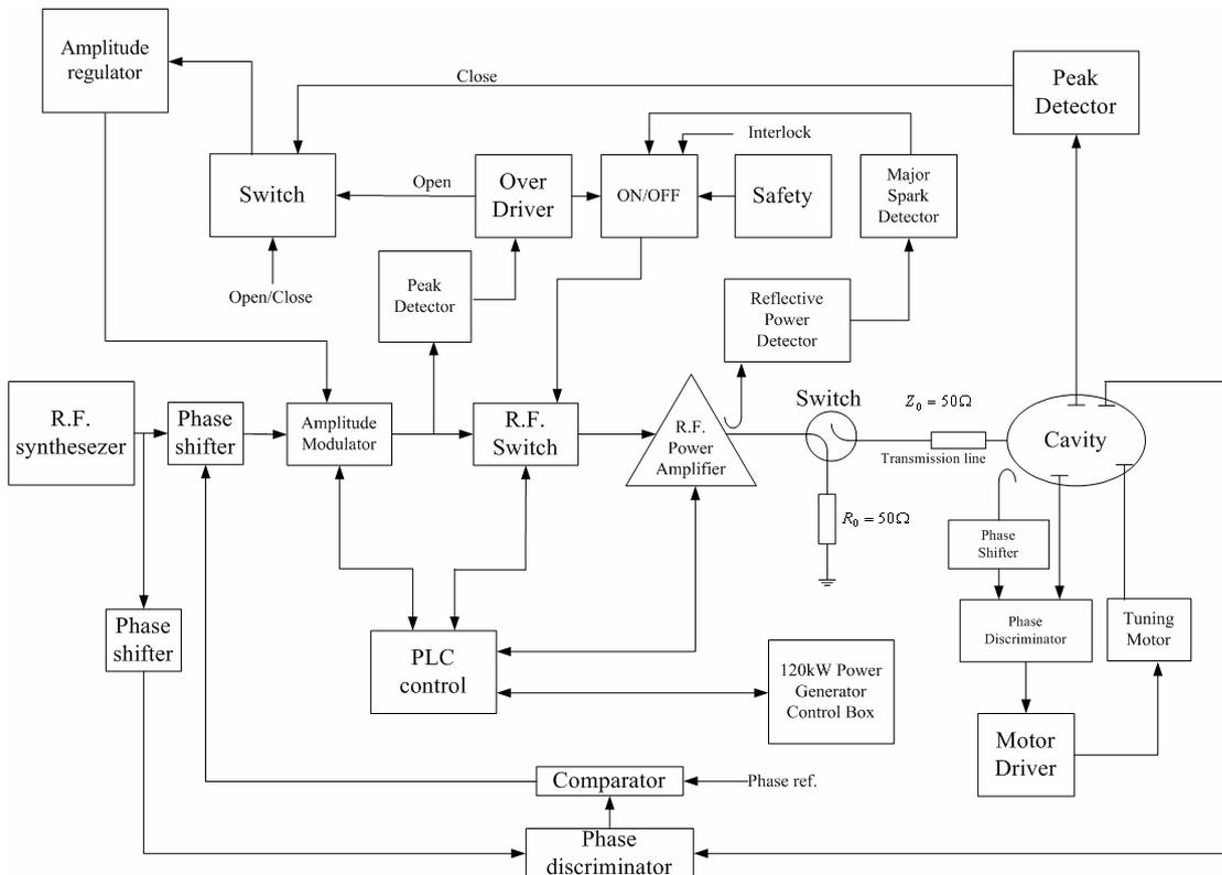
Figure 1: The block diagrams of the R.F. system.
