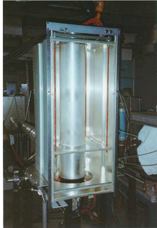
Figure 4: the internal view of final stage amplifier
