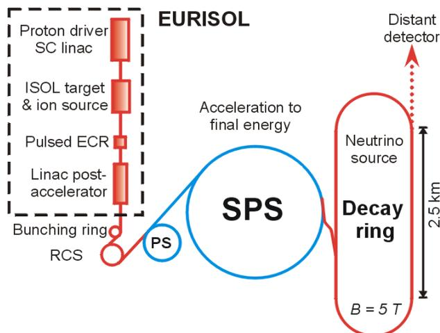
Figure 12: The “beta-beam” concept, illustrated here by coupling EURISOL to the CERN PS and SPL rings.
