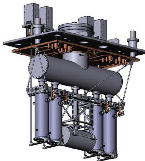
Figure 3. A sketch of the internal components of a medium beta cryomodule. Each of the five medium-beta cryomodules contains two superconducting niobium quarter-wave resonator-cavities on either side of one superconducting solenoid.
