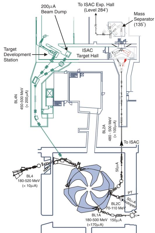
Figure 4. The BL4 cyclotron extraction port will be used to provide beams for high-power target development in an underground expansion of the ISAC target hall (shown in green).
