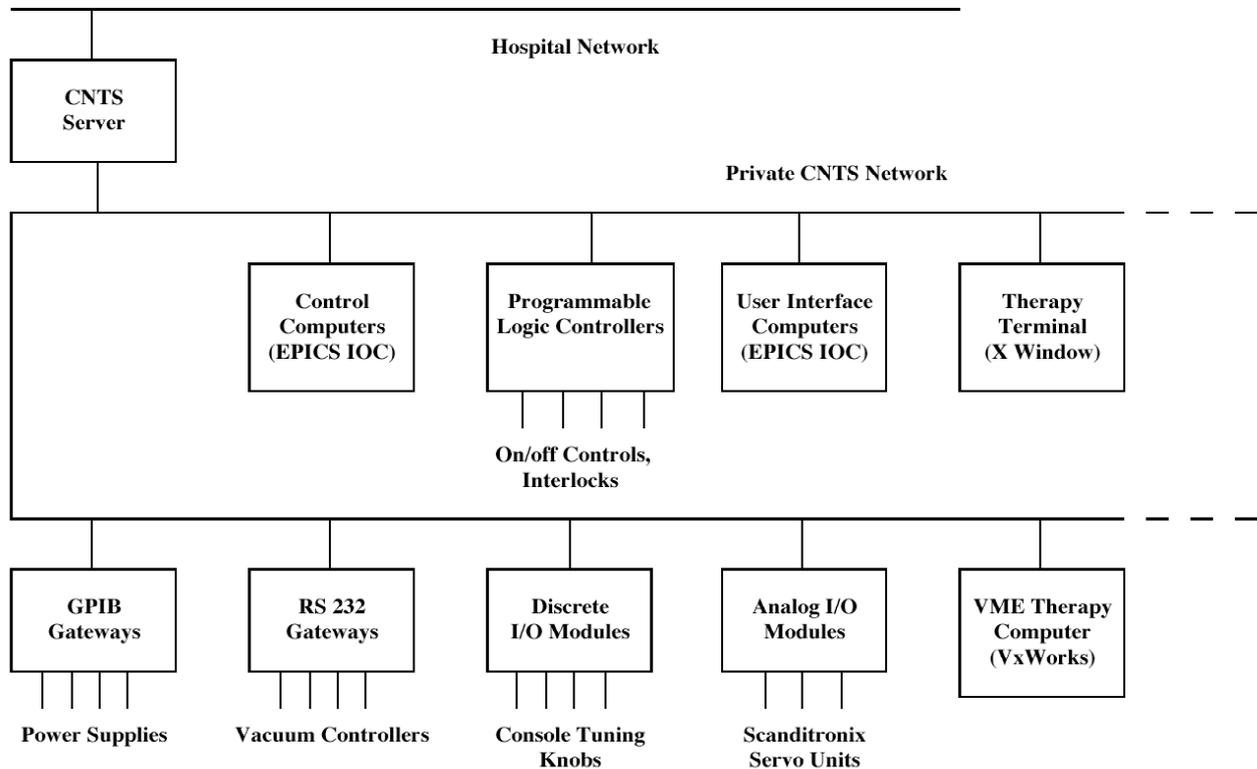
Figure 1: Diagrammatic overview of the control system layout. The gateways and I/O modules are physically located close to the connected equipment and the network acts as a field bus.
