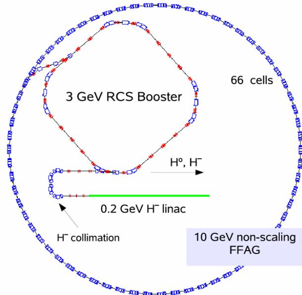
Figure 1: Layout drawing of the 4 MW, NFFAG driver.
